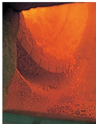
Figure 18.7 The production of CaO from CaCO 3 in a rotatory kiln.
